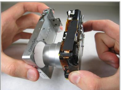
To remove the front cover, gently hold the inside structure of the camera and slowly pull the front cover off.
