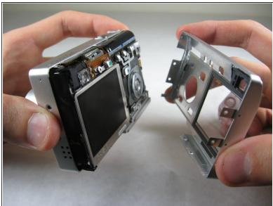
Carefully pull the back of casing away from the front.
