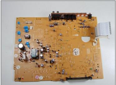
• Lift board up and out of the lower case
