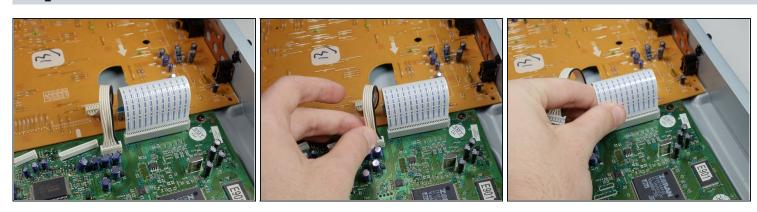
• Disconnect the wires and ribbon by pulling them out of their respective connections
