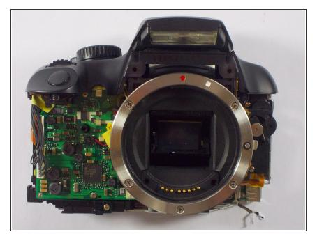
Remove the five silver screws from the lens mounting ring using a Phillips screwdriver.
