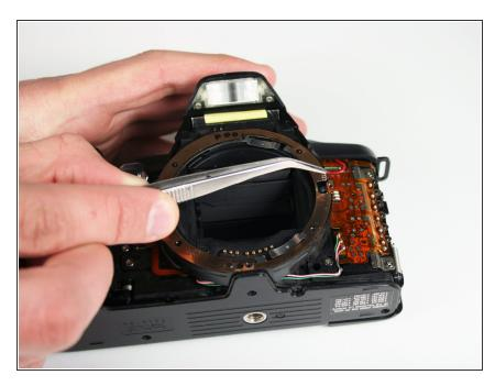
Use a pair of tweezers to remove the spring on the lens mounting ring.
