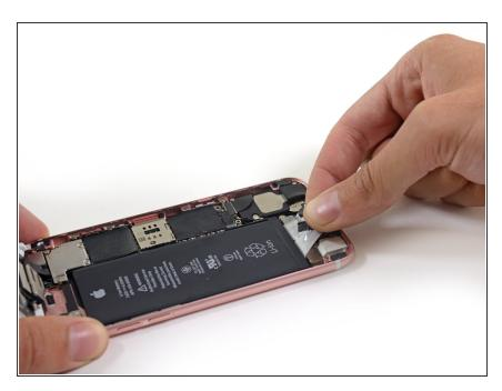
Grab the ends of the two adhesive strips and hold them together. Try to keep the strips flat and wide.
