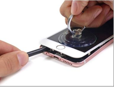
Twist the spudger to open the gap more and break it free from the adhesive.
