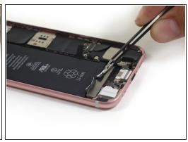
Use tweezers to peel up the edges of the two adhesive strips at the bottom of the battery.
