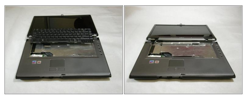
• After the ribbon has been detached, carefully remove the keyboard.
