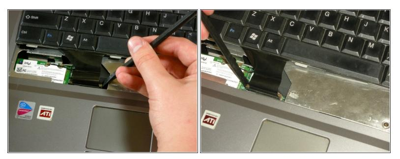
• Use a spudger to release the ribbon cable from the motherboard.
