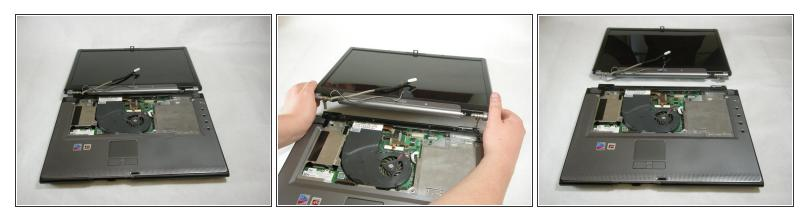
• Hold down the body of the computer by placing your hands in the pictured positions. Then, lift the display from the body.
