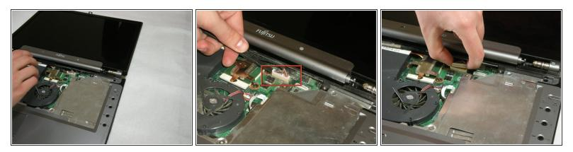
• Use a spudger to detach and remove cables from the motherboard.
