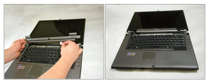
• Disconnect the ribbon cable from the motherboard and remove the hinge cover from the computer.
