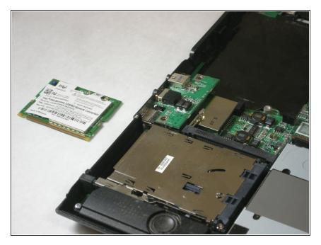
• A picture of the removed wireless module is shown to the left.
