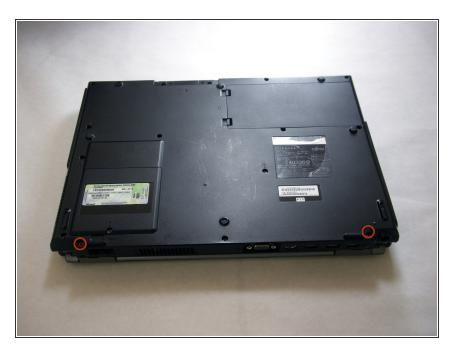
• Remove the screws from the bottom of the hinge as shown in the image.
