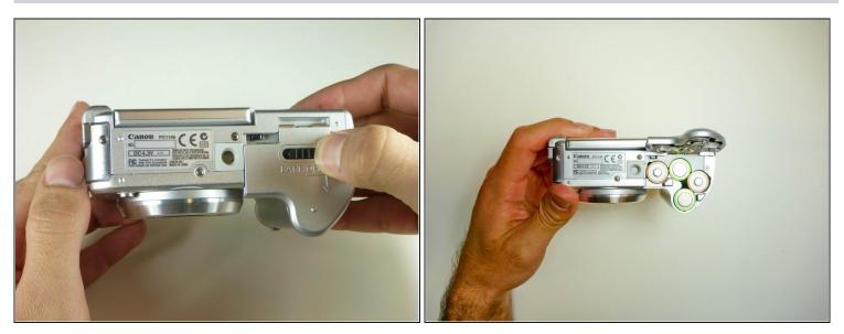
• Unlock the battery cover, while swinging the cover outward to open it.
