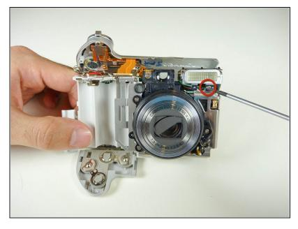
Remove the 3 mm screw that holds the flash unit to the camera.
