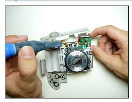
Remove the 3 mm screw that sits on the back of the circuit board.
