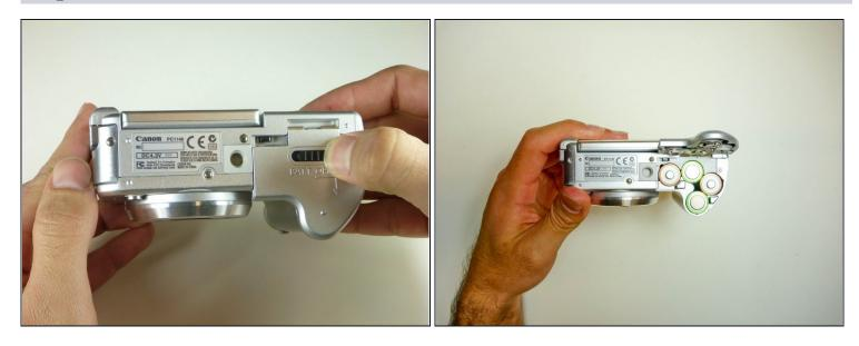
• Unlock the battery cover, while swinging the cover outward to open it.
