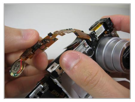
Slowly bend the speaker's wire tape away from the lens assembly. Avoid creasing the tape.
