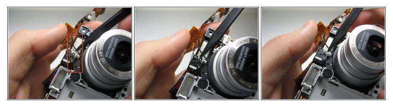
Insert the point of a spudger underneath the wire shown.
