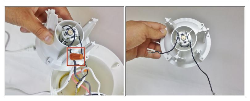
Remove the orange twist-on wire connector connecting the black wire to the grey wire.
