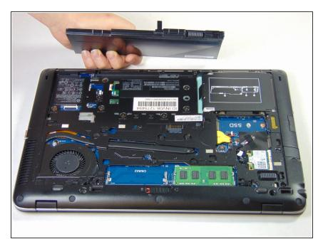
Battery should easily be lifted up and out.
