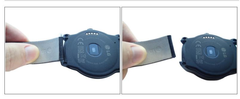
• Once the spring bar is released, pull out the other end to detach the strap.
