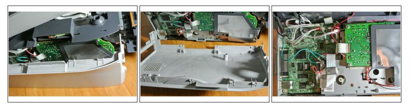
• After you fully removed the cover, you'll have a view on the motherboard, the cable and the plugs.
