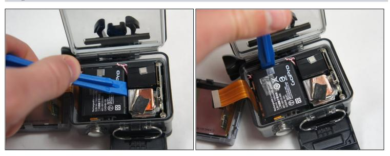
• Place the plastic opening tool at one of the edges of the battery then pry until the battery is removed from the GoPro.
