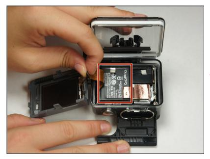
Peel back the rear panel ribbon cable that is adhered to the battery until it is completely separated from the battery.
