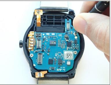
Remove three 3.0 mm Phillips screws on the edges of the motherboard with a Phillips #000 screwdriver.
