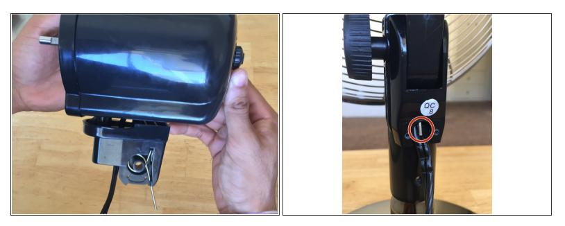
Align the end of the metal coil into the same hole the black wire comes out of in the black cover from step 6.
