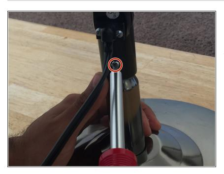
Working with the Phillips #2 screwdriver, loosen the 1/4" center hinge screw from the metal base.
