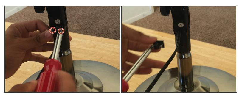
• Using the Phillips #2 screwdriver, separate the wire holder from the back of black cover by removing the two 1/8" screws.
