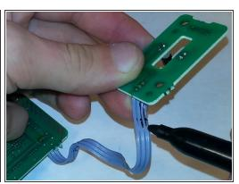
Mark the wire connected to the small circuit board so for future reference.
