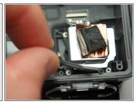
• Remove the two 4 mm Phillips #000 screws securing the top button.
