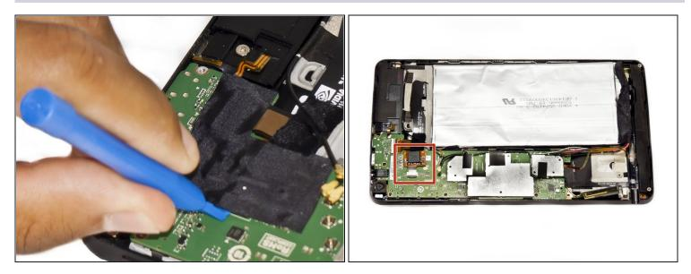
• Peel away the tape covering the top right side of the motherboard. The plastic opening tools are useful in nudging the tape off.
