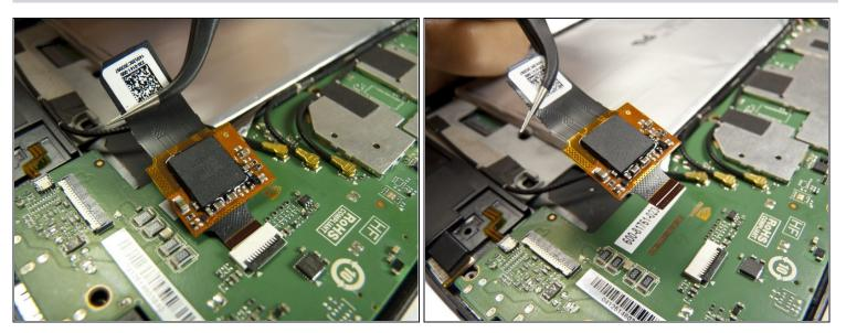
• Using the precision tweezers, gently remove the touchscreen controller from its port.
