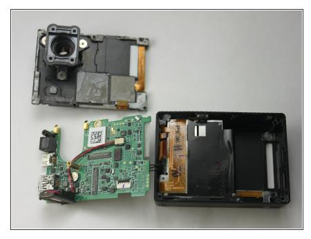
Once the camera assembly has been removed, you can begin separating the motherboard assembly from the camera housing.
