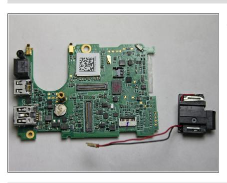
Once disconnected from the motherboard, the speaker assembly can be removed.
