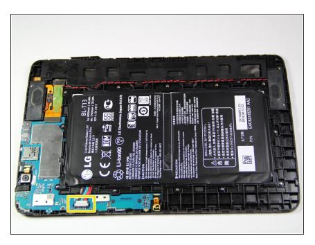
Disconnect the battery by inserting the point of a spudger underneath the white tabs on either side of the connector and gently pry up.
