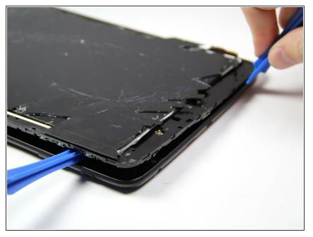
Insert another plastic opening tool (or a similar tool) between the screen and the back panel on the opposite side of the device to hold it open.
