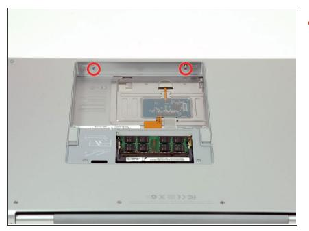
Remove the two Phillips screws in the battery compartment near the latch.
