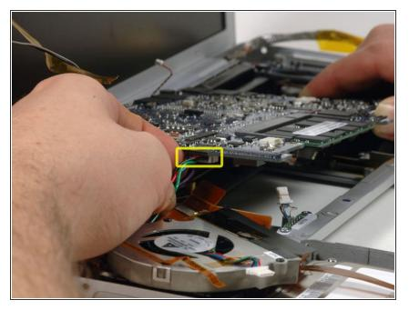
• Lift up the left side of the logic board and disconnect the multi-colored power cable from the bottom of the board.
