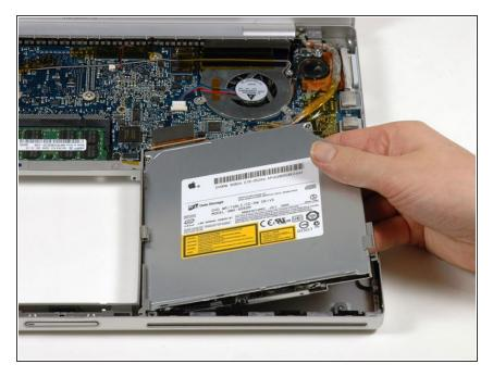
• Lift the optical drive up and out of the computer.
