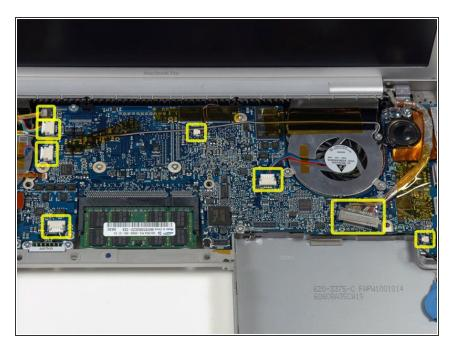
• Disconnect the eight indicated connectors from the logic board, removing tape as necessary.
