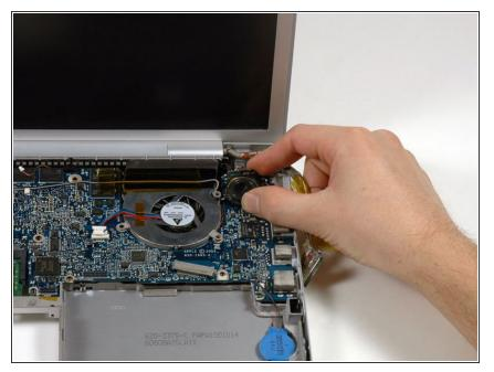
• Rotate the speaker clockwise approximately 30 degrees until it comes free from the logic board.
