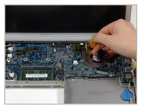
• Peel up the gray and black speaker wires from the top of the logic board, removing tape as necessary.
