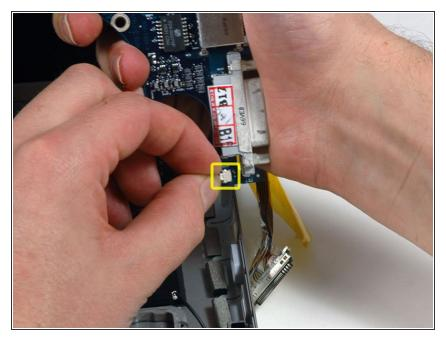
Disconnect the right thermal sensor cable from the bottom of the logic board near the DVI port.
