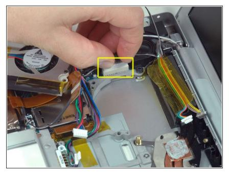
Disconnect the large multi-colored battery connector cable from the left I/O board.
