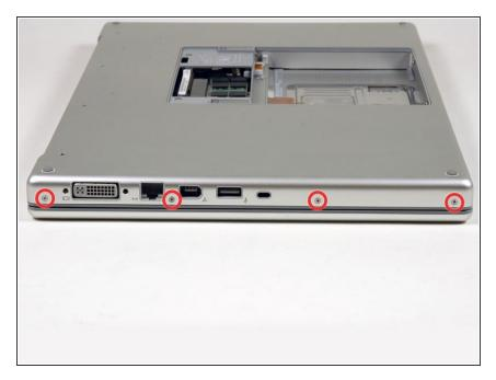
• Remove the four Phillips screws on the port side of the computer.
