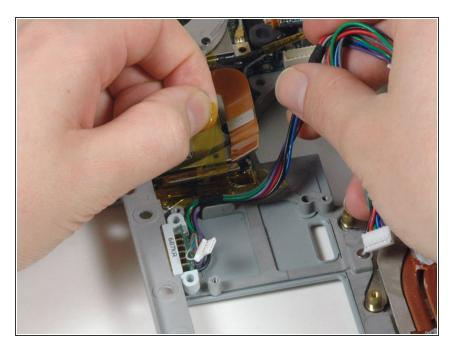
• Peel up the orange tape securing the battery connector to the lower case, and lift the battery connector out of the computer.
