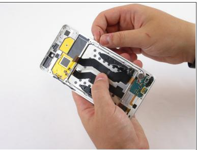
Use tweezers to pull upwards and detach the microphone wire that connects the motherboard to the dock connector.
