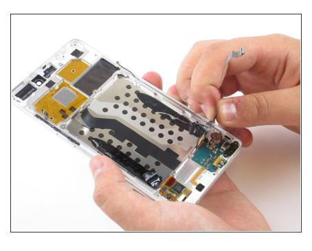
Peel back the ribbon that is adhered to the metal surface as shown.
