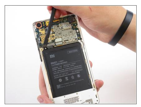
Use a nylon spudger to pry upwards to detach the ribbon that's connecting the battery to the motherboard.
