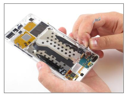
Peel back the ribbon that is adhered to the metal surface as shown.
