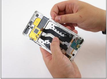
• Use <u>tweezers</u> to pull upwards and detach the microphone wire that connects the motherboard to the dock connector.
