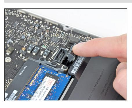
Bend the battery cable slightly away from its socket on the logic board so it does not accidentally connect itself while you work. To reassemble your device, follow these instructions in reverse order.
