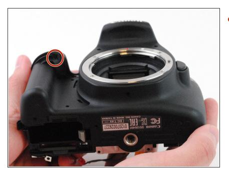
Remove the black 5 mm Phillips #000 screw, located under the grip.
