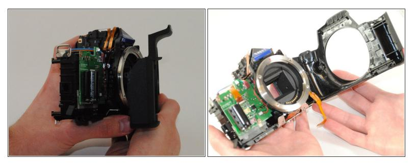
• Remove the front panel of the camera.
