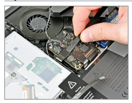
Use the flat end of a spudger to pry the optical drive connector up from its socket on the logic board.
