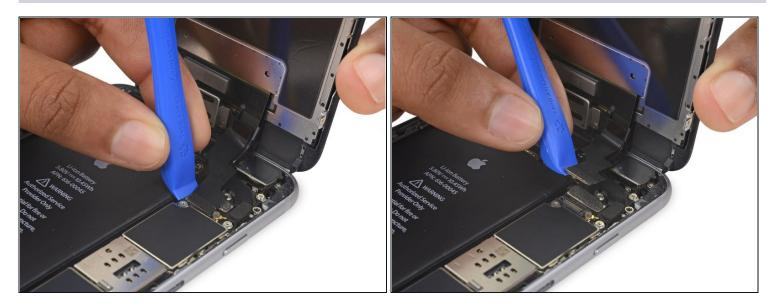
$\triangle$  Be careful to only pry up on the connector itself and not the socket on the logic board.
