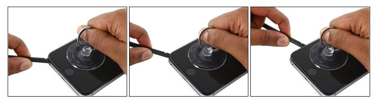
• While firmly pulling up on the suction cup, slide the edge of the spudger under the bottom left corner of the display.
