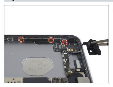
Remove the three 2.4 mm Phillips screws over the audio control cable bracket.
