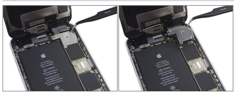
• Remove the display cable bracket.
