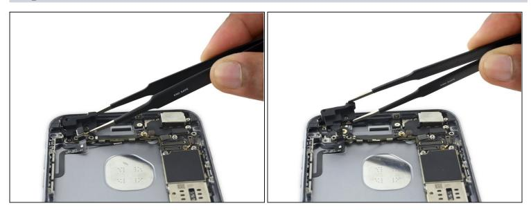
• Lift, but do not remove, the cellular antenna to reveal the third screw securing the audio control cable to the rear case.
