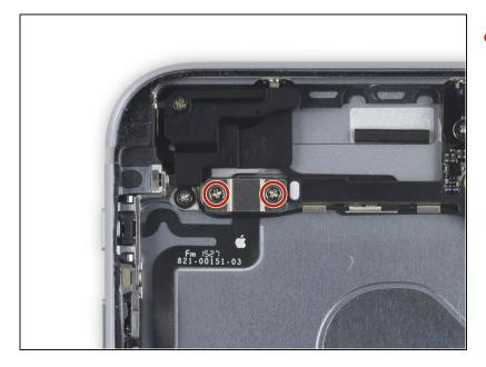
Remove the two 2.7 mm Phillips screws over the audio control cable bracket.
