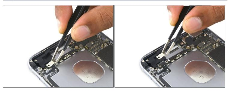
• Remove the audio control cable bracket.
