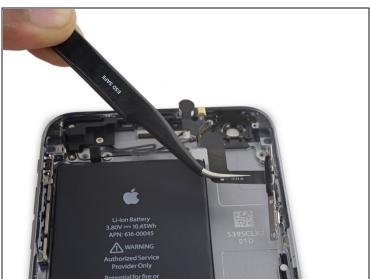
• Remove the power button flex cable.
