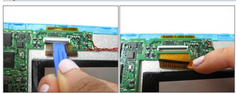
Remove the orange data display ribbon wire above the battery by prying open the ZIF connector with the plastic opening tool.
