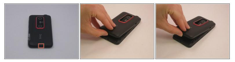
• Remove the outer casing of the phone with your hands by prying and lifting at the latch.
