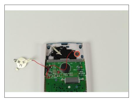
Use the #00 Phillips screwdriver to remove the one 3mm Phillips screw holding the solar panel in place.
