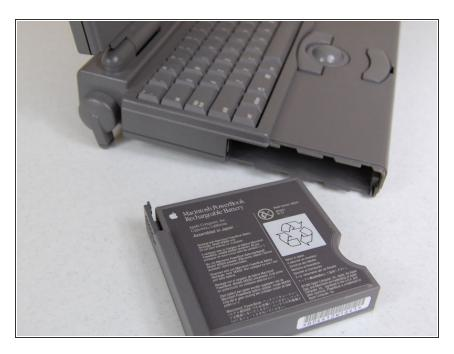
Slide the battery panel ( or switch, depending on the battery) on the left side of the computer so the battery is in the "Unlocked" position. Pull the battery straight out. Put in the new battery and slide the panel/switch to the "Locked" position.
