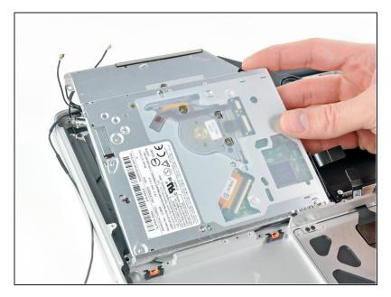
• Lift the optical drive from the edge nearest the display and remove it from the upper case.
