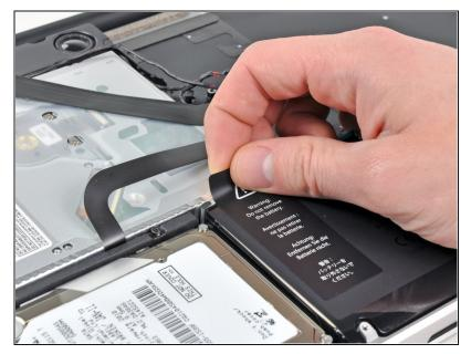
• Carefully peel the battery warning label off the upper case between the battery and the optical drive.
