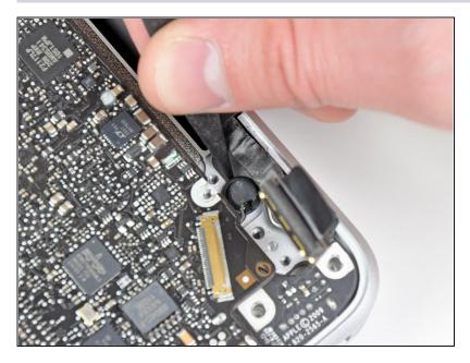
• Use the tip of a spudger to gently peel the microphone off the adhesive securing it to the upper case.
