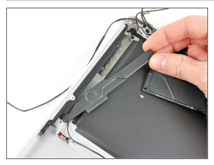
Pull the right speaker out from under the optical drive opening.
