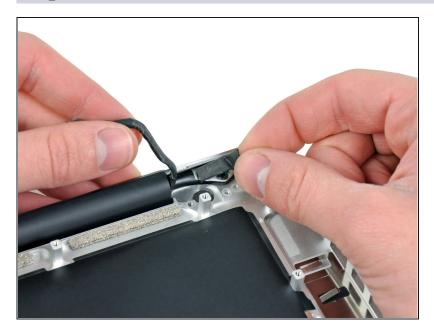
• Remove the small piece of foam tape covering the left display hinge screws.
