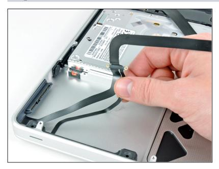
• Carefully peel up the thin IR sensor/sleep LED ribbon cable from the adhesive securing it to the upper case.
