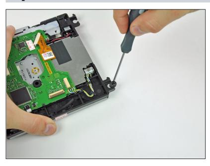
Repeat the procedure described in the preceding step for the second rubber grommet on the rear of the DVD drive housing.
