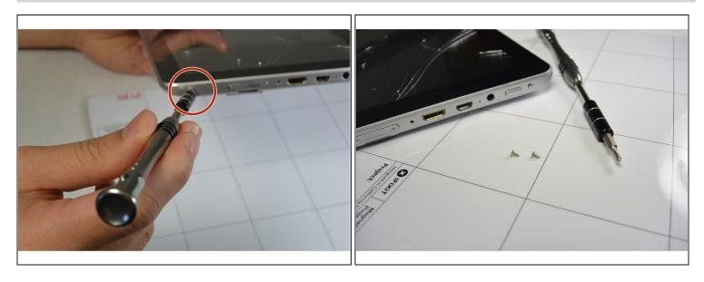
• Remove the two screws from the end of the device where the ports are located using a Phillips #1 screwdriver.
