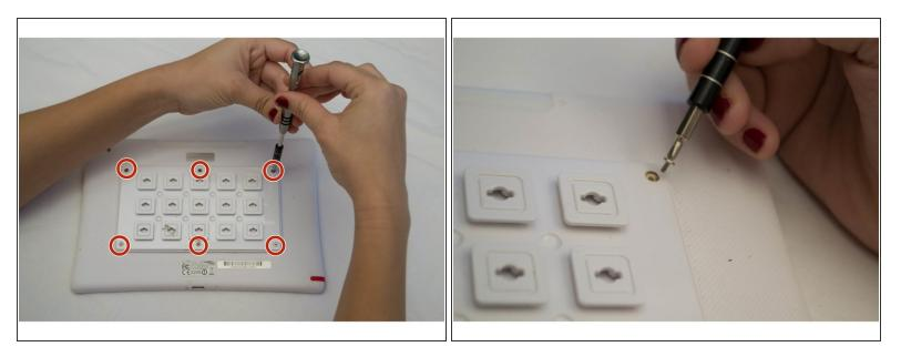
• Remove the six 2.5 mm JIS #000 screws attaching the custom grid to the back panel.
