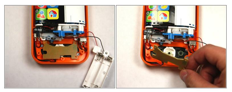
• Carefully remove the button board to gain access to the buttons.
