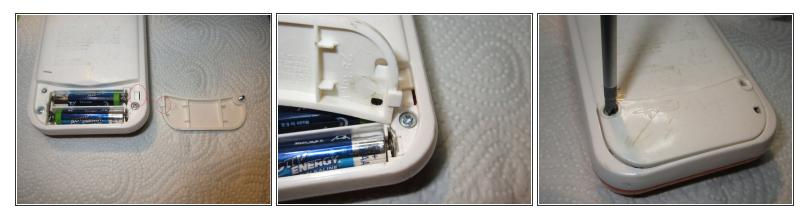
When reassembling, align the notch on the battery panel with the slot on the phone.
