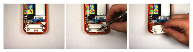
Removed 1 4.8mm phillips head screw with a #0 Phillips head screw driver and lift away battery back being conscientious of wires.
