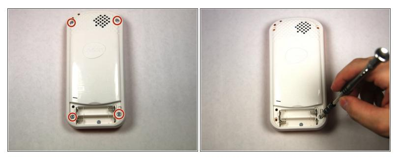
Remove 4 13.8mm screws holding the device back using a Phillips #1 screw driver.
