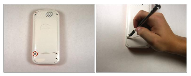
Using a Phillips #1 screwdriver, remove the 4.8mm screw on the battery cover by twisting the screwdriver counter-clockwise.
