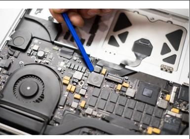
Using the flat end of a spudger, pry the trackpad connector.
