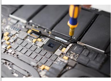
Remove the following T5 Torx battery screws.
