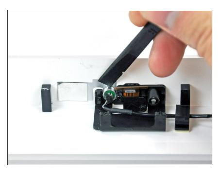
Use the flat end of a spudger to pry the microphone off the adhesive holding it to the front bezel.
