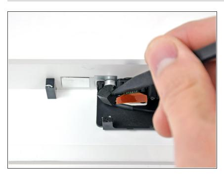
Use the tip of a spudger to remove the foam bumper covering the microphone.
