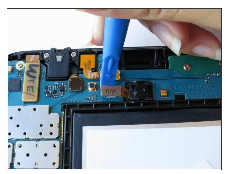
Slightly apply pressure and move the blue plastic opening tool downwards to pop the back camera's metallic rectangular connector from its socket on the logic board.
