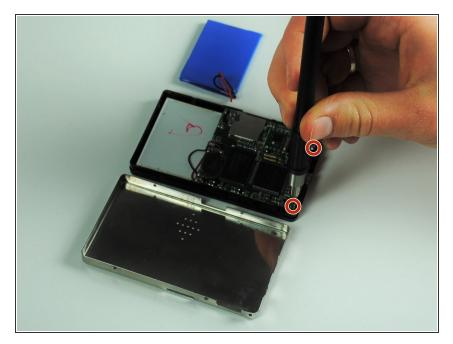
Unscrew the visible Philips head screws (size: 3.968 mm) on the motherboard located on the top of left and right sides. Use a PH #0 sized screw driver head for removal.
