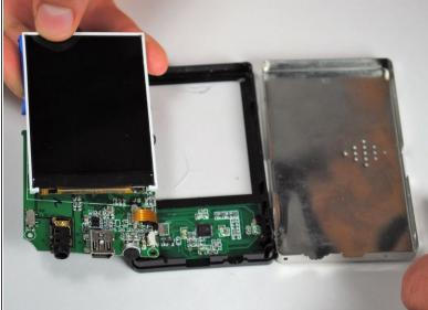
Carefully bend the plastic frame to remove the motherboard.
