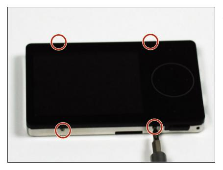
Unscrew the four screws (size: 3.175mm) on the left and right side of the Element Electronics GC-1020 device using the PH#0 screwdriver.
