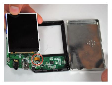
The display is attached to a dark yellow, flimsy, plastic material. This material is then attached to the motherboard. Tear off the plastic, successfully detaching the motherboard and display from each other.
