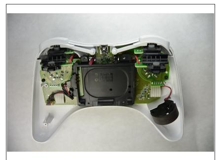
Once all of the screws are removed, simply use one hand to hold the front panel in place and lift up on the back panel to remove it. Place the back panel so the insides are facing up towards you.
