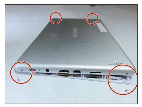
Remove the 4 exterior screws using a <u>Phillips #000 Screwdriver</u>.
