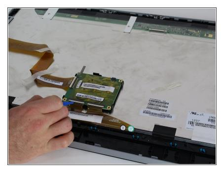
Use a plastic spudger to unclip the 3 ribbon clips on the back of the display.
