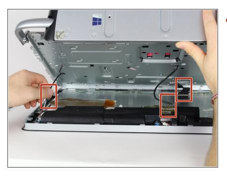
Lift up the computer by the base very slowly, and disconnect the three wired connections to the display with your hands. Always disconnect wired connections from the plastic base.
