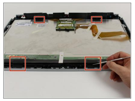
Set the computer aside, and use a small knife to cut the strips attaching the display to the digitizer.
