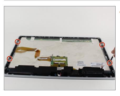
Remove the four 7mm T15 silver screws from the edge of the computer.
