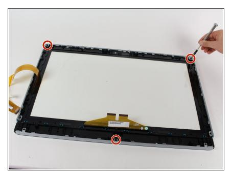
Remove the three 10mm T15 screws from bezel.
