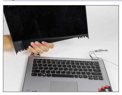
Once the screen is completely free from the rest of the computer, you are able to remove and replace it.
