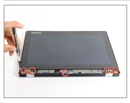
Using a Philips 00 Screwdriver, remove the nine screws of varying sizes that connect the screen to the rest of the computer (four near each of the hinges, one in the center)
