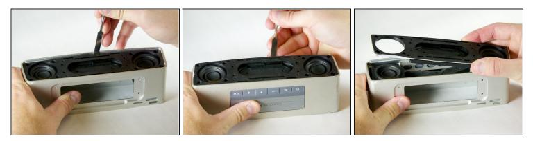
• Using a nylon or metal spudger, pry up the plastic divider and remove it.
