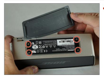
Peel back the rubber battery cover and remove the four circled 6.0 mm screws using a T8 Torx Screwdriver.
