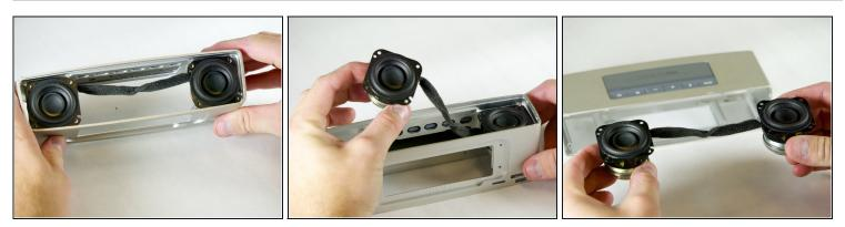
• Gently lift the speakers up and out of the casing.
