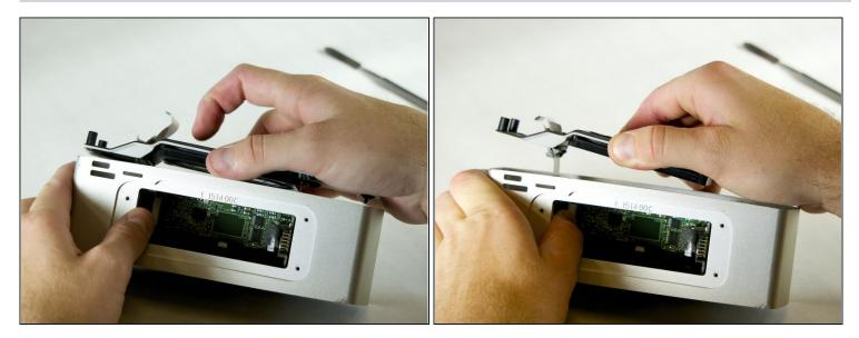
• When removing the plastic divider be careful not to damage the wire strip sliding through it.
