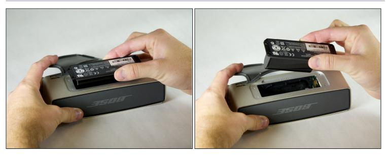
• While holding the cover back, pull straight up on the battery to remove it.
