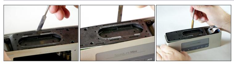
• Use a Metal Spudger to pry up the plastic divider.
