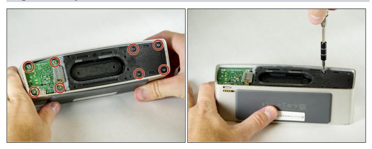
• Remove the four 15.0 mm screws on the left and the four 9.0 mm screws on the right using the T8 Torx Screwdriver.
