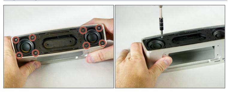
• Remove the eight 9.0 mm screws using the T8 Torx Screwdriver.
