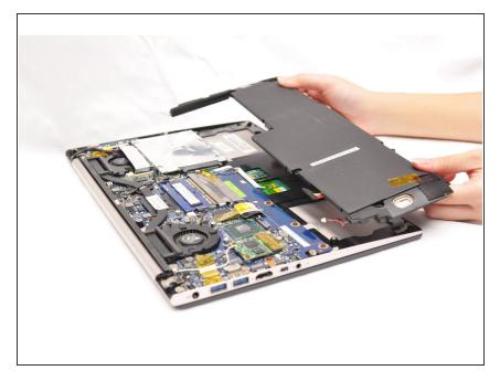
Remove the battery completely.
