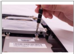
Remove the four 3mm hard drive screws with a <u>Phillips #0 Screwdriver</u>.
