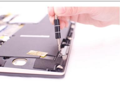
Remove the eight 3 mm Phillips #0 screws on the bottom panel.
