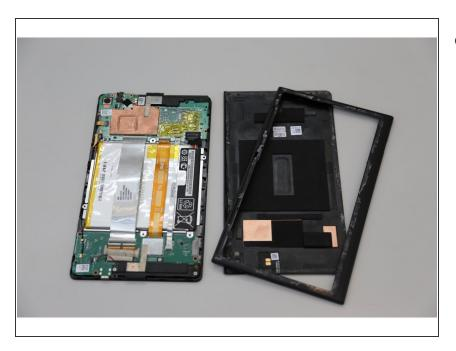
When you take the rear panel and the frame out, place the rear panel and the frame away from the device.
