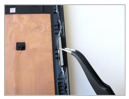
Using a precision tweezer, detach the clear plastic wire from the back casing by pulling the wire out of its slot.
