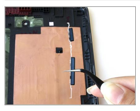
Grab the power/volume button with a precision tweezer to completely lift the buttons out of the back casing.
